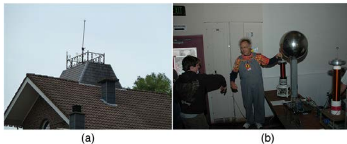
Figure 18.37 (a) A lightning rod is pointed to facilitate the transfer of charge. (credit: Romaine, Wikimedia Commons) (b) This Van de Graaff generator has a smooth surface with a large radius of curvature to prevent the transfer of charge and allow a large voltage to be generated. The mutual repulsion of like charges is evident in the person's hair while touching the metal sphere. (credit: Jon 'ShakataGaNai' Davis/Wikimedia Commons).
