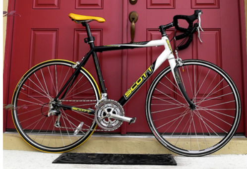
Figure 10.32 The image shows a side view of a racing bicycle. Can you see evidence in the design of the wheels on this racing bicycle that their moment of inertia has been purposely reduced? (credit: Jesús Rodríguez)
